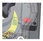
Close the housing of the controller, buckle up the snap joint.
